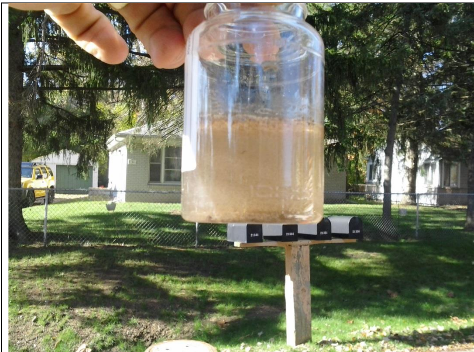
Sample from MH 6240 (269) @ 21351 Seminole. Sample from MH, Toilet paper, grease, and sanitary debris
